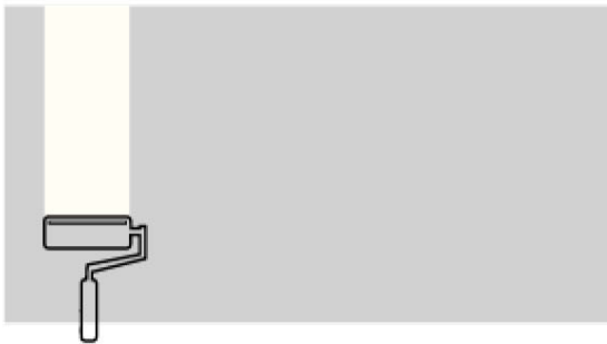
1. Apply adhesive on base surface
